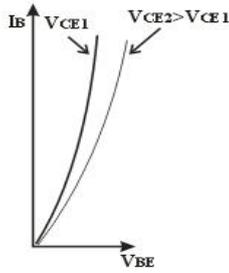
**Input characteristics:** In between input current  $I_B$  and base-emitter voltage  $V_{BE}$ .
