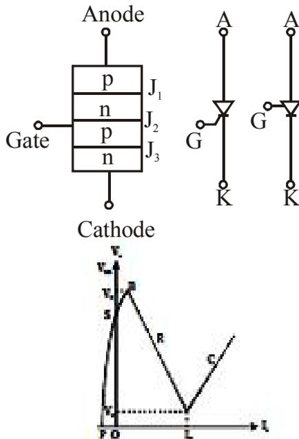
A thyristor has characteristics similar to a thyratron tube. A thyristor (a pnpn device) belongs to transistor (pnp or npn device) family. The name 'thyristor', is derived by a combination of the capital letters from THYRatron and transISTOR.
