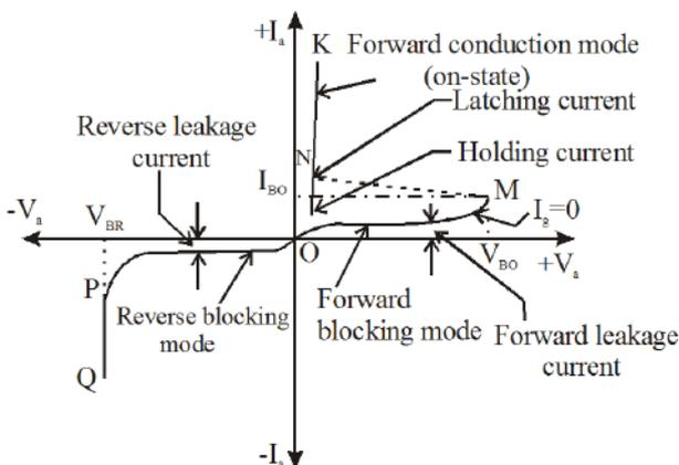
**Forward blocking mode:** Junctions  $J_1$ ,  $J_3$  are forward biased but junction  $J_2$  is
