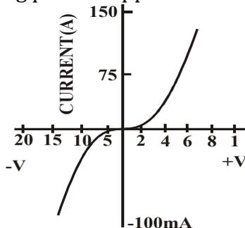
In a Schottky diode, only electrons participate in the conduction mechanism unlike in p-n junction diodes because there are no holes in the metal. As a result, there is no minority carrier storage decreasing the recovery
