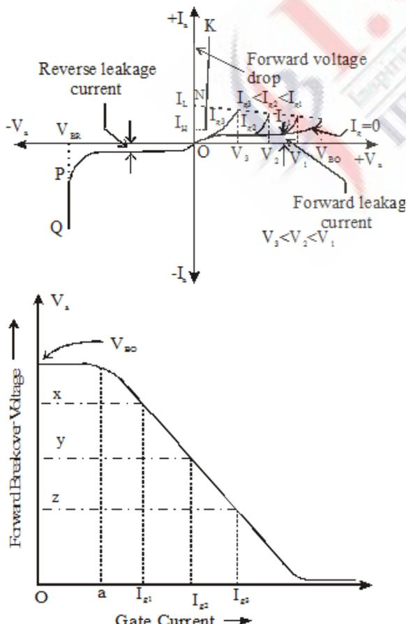
**3. With forward voltage across the anode and cathode** of a thyristor, the two outer junction  $J_1, J_3$  are forward biased, but inner junction  $J_2$ , has the characteristics of a capacitor due to charges existing across the junction. In other words, space-charges exist in the depletion region near junction  $J_2$  and therefore junction  $J_2$  behaves like a capacitance. If forward voltage is suddenly applied, a charging current through junction capacitance  $C_j$  may turn on the SCR.
